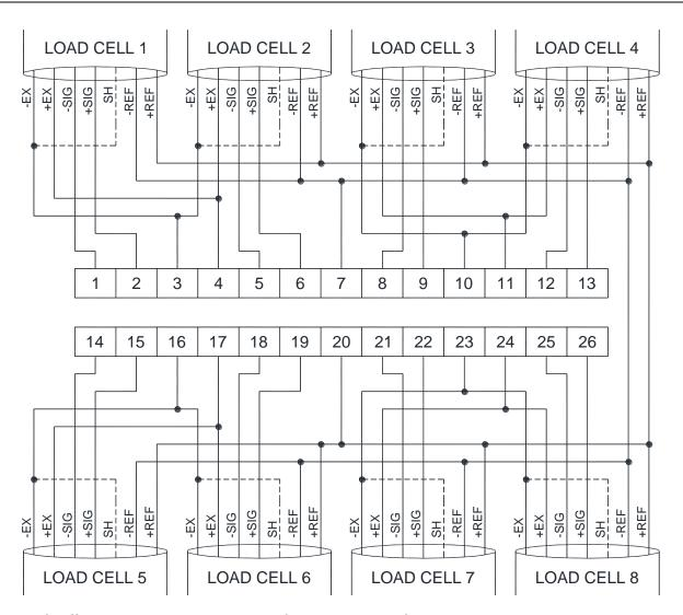
In case of difficulty connecting all the reference wires of the installed load cells, simply connect those of the load cell located at the average distance from the instrument. The reference wires not used must be individually isolated.
